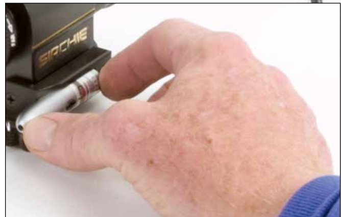
FIGURE 1 —Snap the Laser Pointer into the mounting cradle located on the left side of the Imager.
