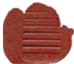
Tool mark left behind in wood is cast using the brown compound of PVS200.
