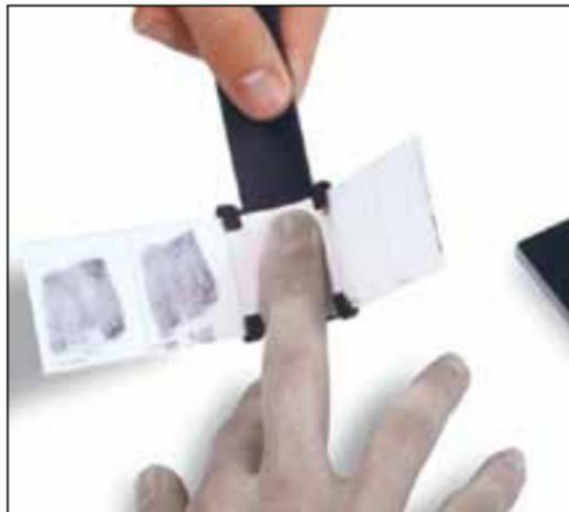
***Gently place the inked finger in the arc of the PMNS60 Record Strip Holder and exert pressure. Do not roll the finger—simply press downward.***
