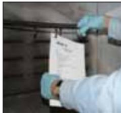
*The document to be treated with NSI609 is secured inside a fuming hood with evidence clips.*
