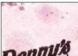
Cash register receipt (left) developed visible prints when tested with NHT609 NinhydrinHT (close-up shown above).
