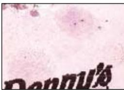
Cash register receipt (left) developed visible prints when tested with NHT609 NinhydrinHT (close-up shown above).
