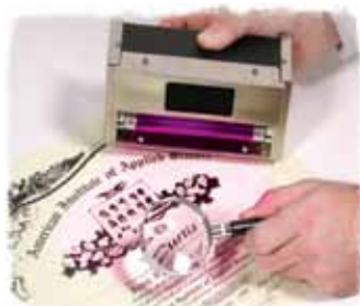
Questioned document examined with No. 782ADC Tiger Twin Dual Wavelength (shortwave/longwave) UV light source and No. 316M Magnifier. Both are supplied with the MQDA500 Kit.
