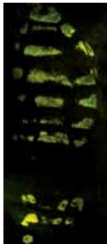
LV517L Acid Yellow on tile with 455nm illumination and viewed through amber filter
