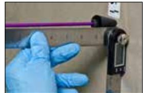
*Note: If the angle of the penetration is measured in reference to the wall, the angle must be recalculated to the floor/ground by subtracting from 90 or 180 degrees depending on the orientation of measurement.*
