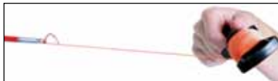
FIGURE 8 —Colored Trajectory String is attached to a Photographic Rod using one of the Stringing Tips.
