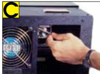
while grasping the lamp. It is recommended that a cloth be used when holding and installing lamps. The lamp will slide out to the side.
