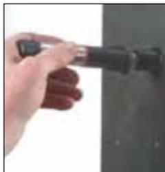
*The upper inlet port on the unit is provided for fuming with the CYANOWAND™. It also supports the PUM100 Portable Humidifier should additional moisture be required.*
