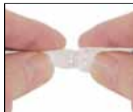
FIGURE 1—Holding the ampoule between the forefinger and thumb of each hand, break ampoule at score.
