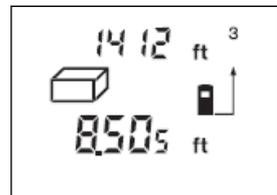
After taking the third measurement, the volume is automatically calculated and displayed. The last individual measured value is indicated at the bottom in the display, while the final result is shown at the top.
