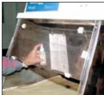
**FIGURE 1—DFO will often produce visible prints using the No. AC632 Forensic Workstation.**
