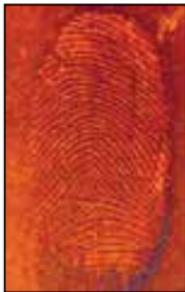
**Use A Barrier Filter**—A barrier filter on the camera is necessary because of the same reason you needed one for your eyes. If you are using standard UV light sources, equip the camera with a filter that is the same color as the goggles used to view the fluorescence.
