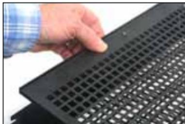
*The DBS3 features a base screen and insert shown on the left. When rotated in 90° increments, the insert creates hole openings measuring from 1/8" to 1/4". The insert is secured by two (2) thumbscrews (shown right). With the insert removed, the sifting screen has a hole opening of 3/8".*
