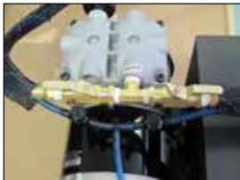
1A. Flow Valve shown in OPEN position.
