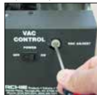
Adjust vacuum level with flathead screwdriver.
