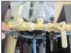
1B. Flow Valve shown in CLOSED position.
