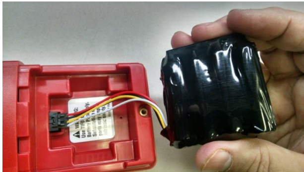
Figure 3: Insert battery pack into case
