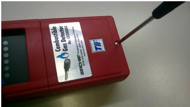
Figure 1: Loosen screw & remove battery cover
