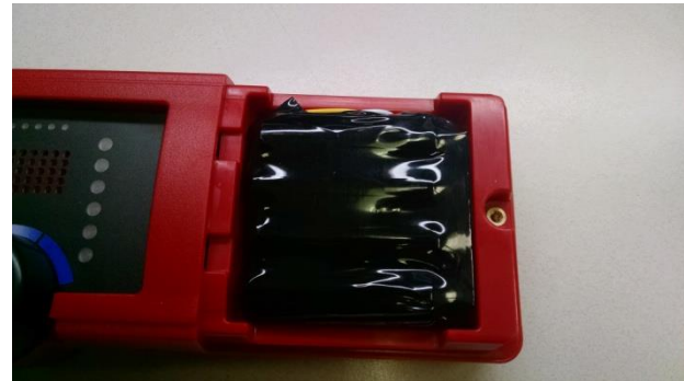
Figure 4: Battery pack correctly installed
