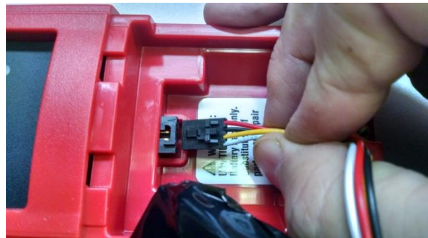
Figure 2: Plug-in the battery connector
