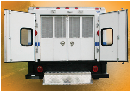
Center Divider with Individually Locking Rear Doors
