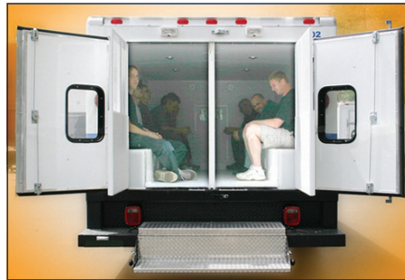
Fold Down Step Accommodates Prisoners with Leg Shackles
