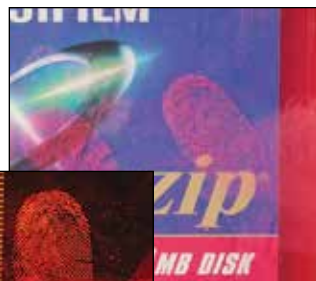
ZIP Disk Case (above) dusted with LL701. Inset (left) photographed with BLUEMAXX™ illumination.
