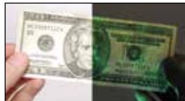
Twenty dollar bill (treated with CLUE SPRAY™) as it appears under normal light (left) and UV light (right).
