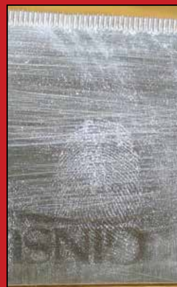
CYANOACRYLATE FUMED knife blade photographed in natural light—print faintly visible.
