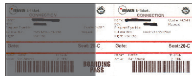
The part of the airline boarding pass sprayed with Special Formula Ninhydrin (NSI609) for prints turns black.
