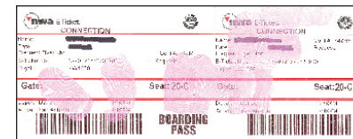
Airline boarding pass reveals an abundance of latent prints when sprayed with NinhydrinHT (NHT609).
