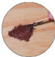
FIGURE 3—Apply the material to the surface to be cast.
