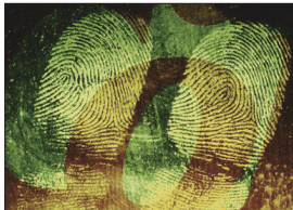
Cyanoacrylate developed latents enhanced with Ardrox fluoresce with BLUEMAXX™ illumination.
