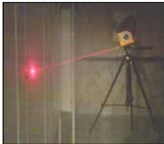
FIGURE 7 —Introduce Photo Laser Smoke (LTF100S) into the scene to make laser beam visible for photos.
