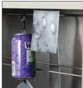
The control prints serve as an indicator for adequate fuming time.
