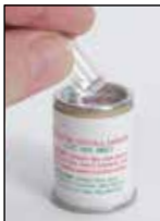
Empty iodine crystals onto metal top of activator canister.
