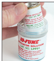
Empty iodine crystals onto metal top of activator canister.
