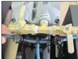
1B. Flow Valve shown in CLOSED position.
