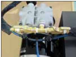
1A. Flow Valve shown in OPEN position.
