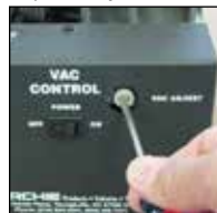
Adjust vacuum level with flathead screwdriver.
