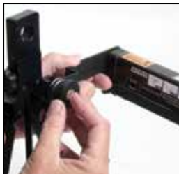
Remove the threaded knobs from the rigid support arms.
