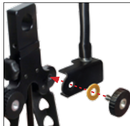
Slip the BTS100UL supports directly onto the body of your BTS100. Secure into place using the fiberglass washers and threaded knobs from the previous supports—the flat steel washers are no longer required.
