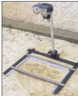
No. UPS100 Universal Photo Evidence Stand is employed to take a photograph of the footwear impression prior to any attempt to cast is made.
