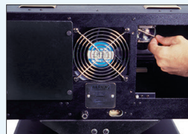
Bulb replacement is simplified with the easy-access rear panel.
