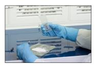
horizontal laminar airflow with dual HEPA filtration.
