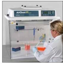
inaccurate, costing the lab technician valuable time and reagents. PCR Workstations minimize this risk by keeping airborne contaminants away from samples and irradiating work surfaces and tools between amplifications.
