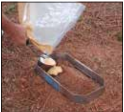
4. Pour mixed casting material into impression.
