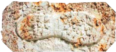
Footwear cast made using casting plaster and adjustable casting frame.
