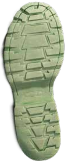
Footwear cast made using SirchTrak Green Dental Stone and Bio-Foam.
