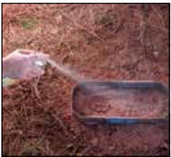
1. Prepare impression with 638CA Dust and Dirt Hardener.
