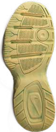
Footwear cast made using SirchTrak Buff Dental Stone and Bio-Foam.
