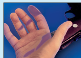
After reagent application and shortwave UV exposure, trace metal is detected.
