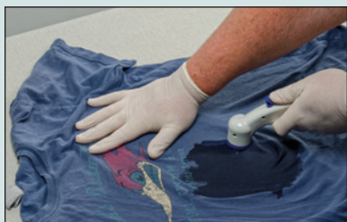
DNA collection of suspected physiological fluids from porous surfaces such as clothing.
