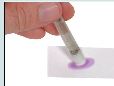
Applying reagent to non-destructive contact transfer.
