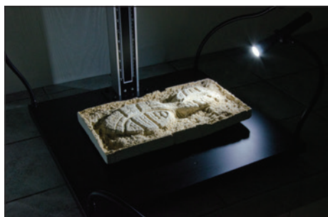
Larger evidence such as footwear castings can be photographed by raising the mounted camera using the column adjustment. The resulting photo is made possible by using the white light from an oblique angle. (camera not included)
