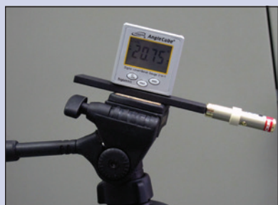
Measure trajectory angle with DMANGLE digital angle finder and laser mounted on tripod using the tripod adapter
