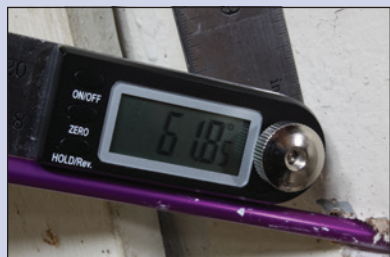
Measure angle of entry with the No. DRP10 digital protractor
