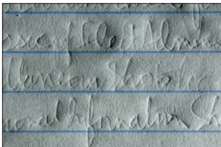
Oblique white light used with a DSLR with macro lens for close-up photos of indented writing. (camera not included)
