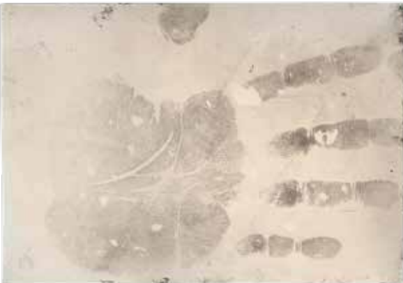
Palm Print developed with black latent print powder, and lifted from a curved plastic surface with GLT101W.
