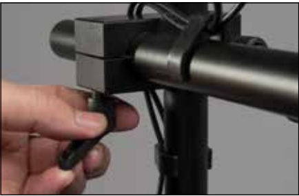
Make precise adjustments to the position of both the KrimeSite™ Imager and the included Shortwave UV light.
