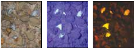
Searching an area littered with small stones (left). Bone fragments are revealed using the 395nm UV Light (middle). Greater contrast with background using Blue 455nm light with orange filter (right).
