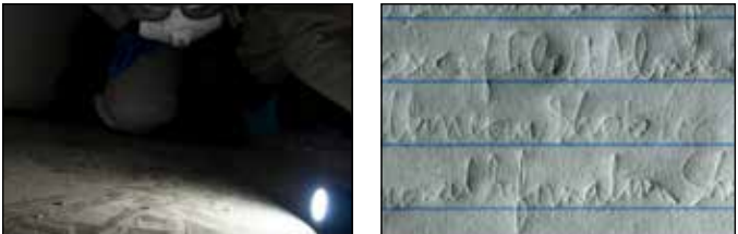
Oblique White light used to reveal Dust Prints on a floor (left) and indented writing on paper (right).
