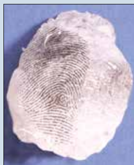
A Liquid Rubber Fingerprint Lift from a highly irregular surface.
