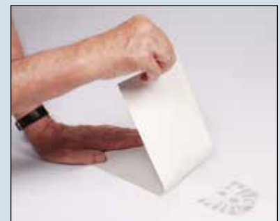
Technician lifting a footprint with the No. GLT401W White GELifter™.
