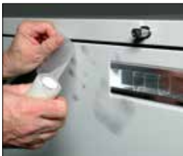
No. 145L4 is used to lift a palm print from a file cabinet.
