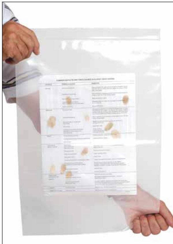
Placing Iodettes in a plastic bag creates an instant fuming chamber.
