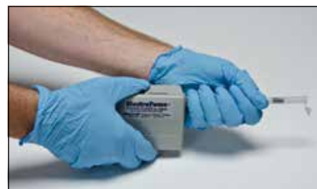
When fuming with this unit, the iodine fuming gun must be warmed by holding it in the palm of your hand.
