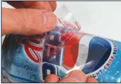
A technician uses Lift-O-Tabs™ to lift a print from a soft drink can.
