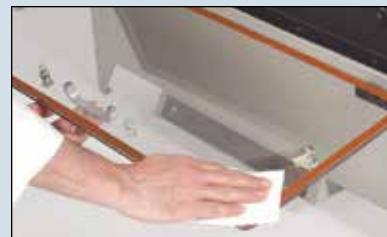
Prior to initial use, treat the inside of the chamber door with Cyano-Bloc™ to protect it from cyanoacrylate buildup.
