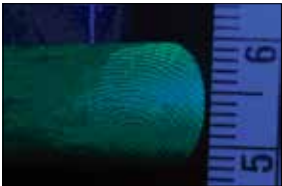
Photo of Ardrox-stained Cyanoacrylate print using 395nm UV light
