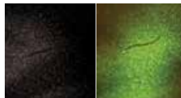
590nm —This single dark blue fiber was located on a black shirt using the 590nm Light. The fiber is not fluorescent, but the background does show slight fluorescence making the fiber stand out against the background as shown right. (Orange barrier filter used for photograph.)
