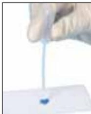
**DISPOSABLE PIPETTES (No. 288DP)**—The disposable pipettes are used to evacuate liquid from one ampoule to the other and as an applicator for the mixed reagent (see photo to the left). To use, simply remove the protective clear plastic cover and either fill or evacuate the pipette by squeezing the plastic bottle.
