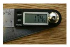
REV: Press <HOLD/Rev> for 3 seconds and the display will reverse.
