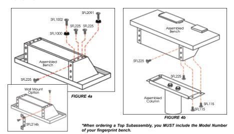
4b. Place the unit in an upright position. Secure the end panels to the back with 6-32 x 1/4" pan head screws and tighten. Place the assembled column on a level surface. Place the bench on top of the column with the front of the bench facing the tabs on the column top. Secure the bench to the column using four 6-32 x 3/8" pan head screws. Secure the end panel to the bottom with two 6-32 x 1/4" pan head screws. Your unit is now ready for use (Fig. 4b).
