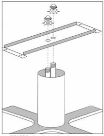
FIGURE B-Attach mounting plate to column.
