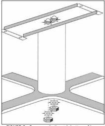
FIGURE C—Secure rods through bottom of base.
