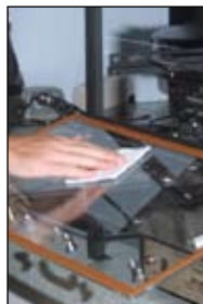
FIGURE 2—CNA110A is applied to the insides of the fuming tank to protect from cyanoacrylate buildup.
