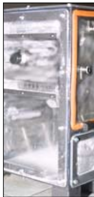
FIGURE 1—Cyanoacrylate buildup on insides of untreated fuming tank.
