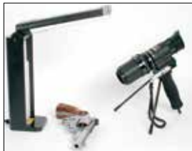
SKSUV13 is paired up with the KRIMESITE™ IMAGER to reveal latent prints on a suspect gun.
