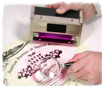
Questioned document examined with No. 782ADC Tiger Twin Dual Wavelength (shortwave/longwave) UV light source and No. 316M Magnifier. Both are supplied with the MQDA500 Kit.
