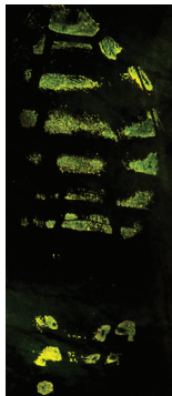
LV517L Acid Yellow on tile with 455nm illumination and viewed through amber filter
